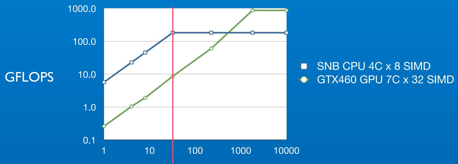
At 32 elements, 183 GFLOPS vs. 8.6 GFLOPS
