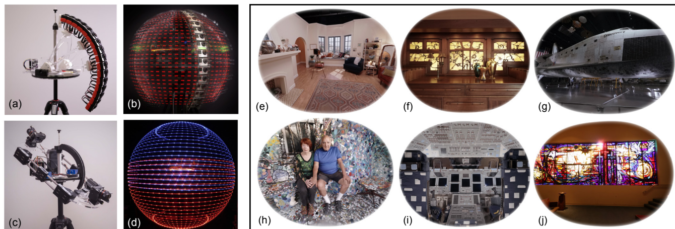
Fig. 1. Acquiring and rendering panoramic light field still images. (a,c) Our two rotating light field camera rigs: the 16xGoPro rotating array of action sports cameras (a), and a multi-rotation 2xDSLR system with two mirrorless digital cameras (c). (b,d) Long exposure photographs of the rigs operating with LED traces indicating the positions of the photographs. (e-j) Novel views of several scenes rendered by our light field renderer. The scenes are: (e) Living Room , (f) Gamble House , (g) Discovery Exterior , (h) Cheri & Gonzalo , (i) Discovery Flight Deck , and (j) St. Stephens .
